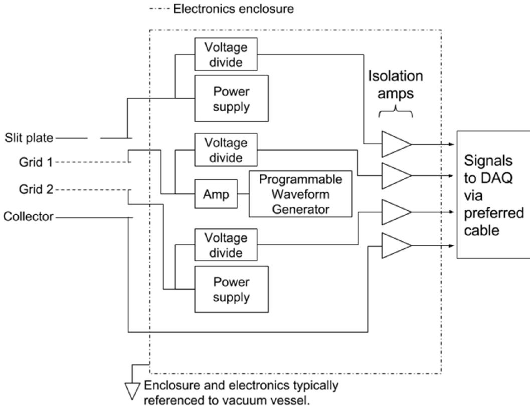
The electronics schematic is shown above for the unidirectional and axial variations; the bidirectional electronics include additional collector and slit plate circuits. The sweep frequency and grid/slit plate potentials are remotely controlled. Potential dividers on the grid/slit plate circuits and isolation amplifiers (circuit shown on right) on all circuits ensure that the data acquisition system is protected.
